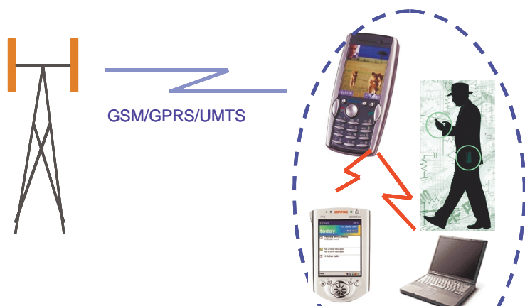
Figure 1 - Seamless access with your phone as the gateway to the public network
