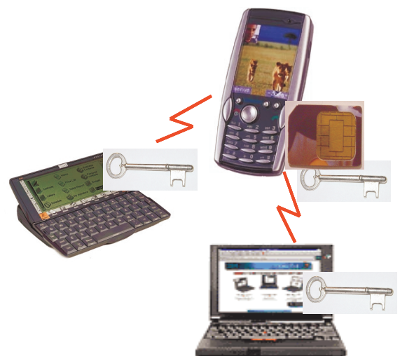
Figure 3 - Authentication and security in your "personal sphere" provided by the SIM
